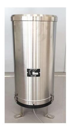
The **WxRG-160** is a Tipping Bucket Rain Gauge and Precision Weather Instrument designed for measuring rainfall. The gauge is shaped like a funnel and features a 204mm diameter screen. When rainwater enters the funnel, it flows into a triangular-tipping bucket. When the water amount reaches 0.2mm, the bucket tips over and triggers a closed reed switch, generating a pulse signal that is sent to a data logger or any other interface.
