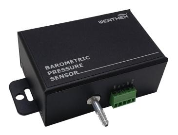
**WxB-101** measures the atmospheric pressure using internal silicon capacitive, Which ensures long-term stability and high accuracy of the pressure measurement. Measured pressure data is collected via RS-232 interface and protocol. It can be used for general purpose use and high precision weather observation.
