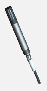
The WxHT-120 is a device used to measure temperature and relative humidity in the air. It features a Teflon filter on the sensing unit, providing high durability against dust and other particles. The device incorporates a capacitive humidity sensor, which offers fast response times and high stability.
